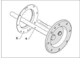
On completion of cleaning, refit all removed parts in the reverse order, taking care to ensure the efficiency of the seals. Position the heater sensor bulb so that it reaches the bottom.
