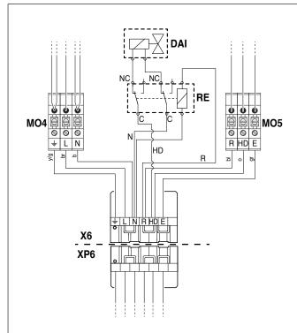
RE Relay (not supplied)MO4 Terminal stripMO5 Terminal strip
