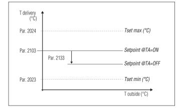
**Mode 4**: operation with variable setpoint according to the value of the input signal 0-10V
